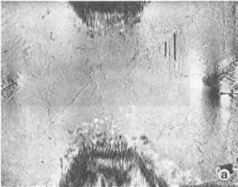
Fig.10: a) X ray topography of D-KDP single crystal with growth defects b) Damage on the TV image electrically stored in the crystal due to the defects
